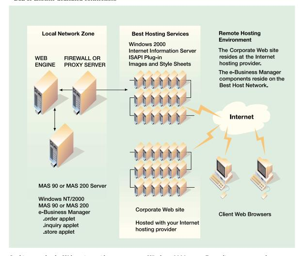
In this example, the Web engine resides on a separate Windows 2000 server. Depending upon network configuration and system load, this component may coexist with MAS 90 or MAS 200 and/or other applications.
